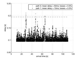
Fig. 3. Results from a single simulation. Circles are packets that arrived from path 0. Crosses are packets that arrived from path 1. X axis is the packet arrival time and Y axis is its delay. The dashed line is the jitter-buffer threshold. In this simulation, PMR = 1 and delay-centric algorithm is active.
